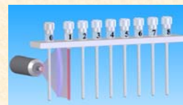
Fig. 2. Configuration of test capillary and LED illumination.
